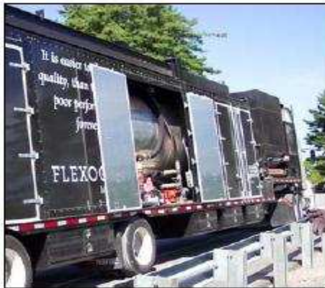
Side view of Polycarb's truck (note resin and catalyst storage tank).
