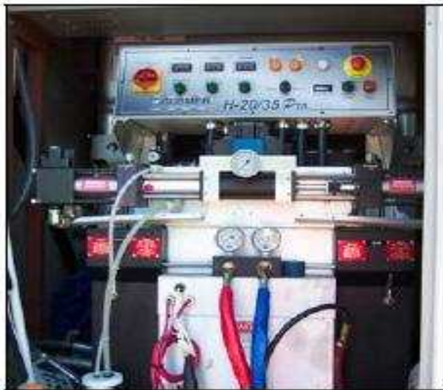
Onboard computerized blending system on Polycarb's truck.
